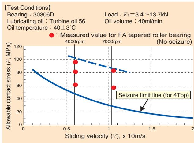
Fig. 5 Contact stress resistance test results
