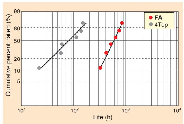
**Fig. 2** Condition ② Results of life test for 30306D
