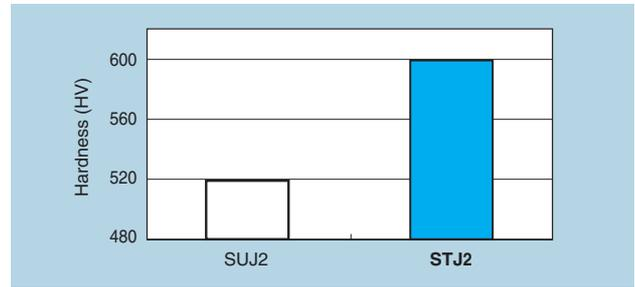
**Fig. 3** Comparison of hardness at temperature 300°C
