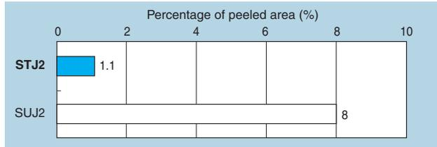
Fig. 7 Peeling resistance test result
