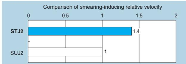
Fig. 8 Smearing resistance test result
