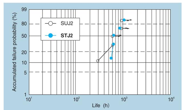
Fig. 12 Fatigue-crack life at high temperature
