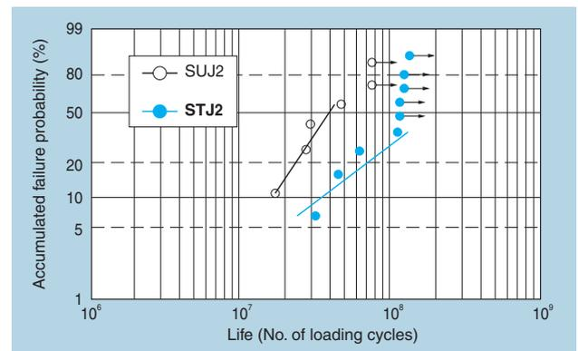
Fig. 11 Fatigue-crack life at normal temperature
