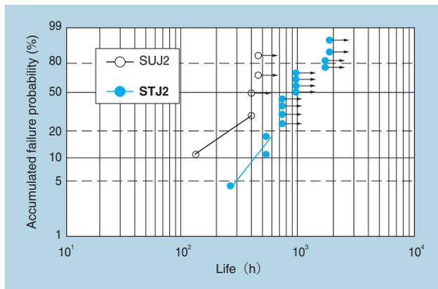
**Fig. 4** Life test result with bearings
