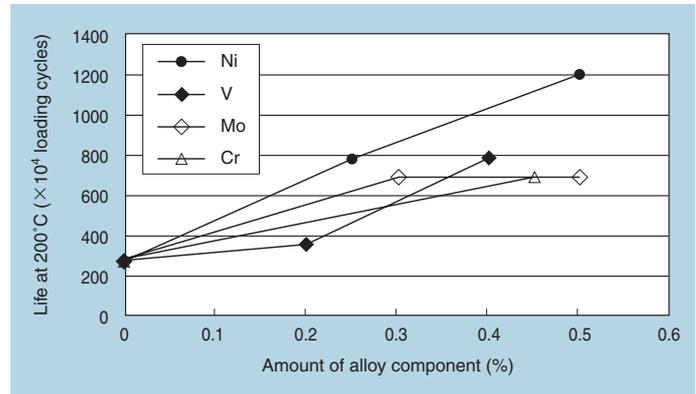
**Fig. 1** Effect of alloy component on rolling life
