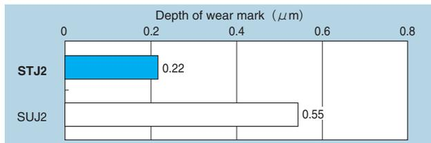
Fig. 9 Wear resistance test result
