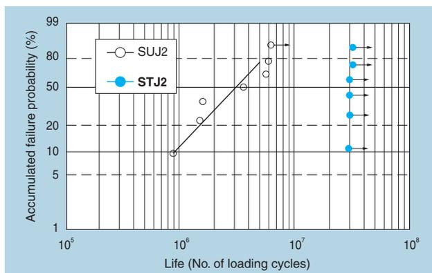
**Fig. 6** High-temperature life test result with thrust-type test pieces
