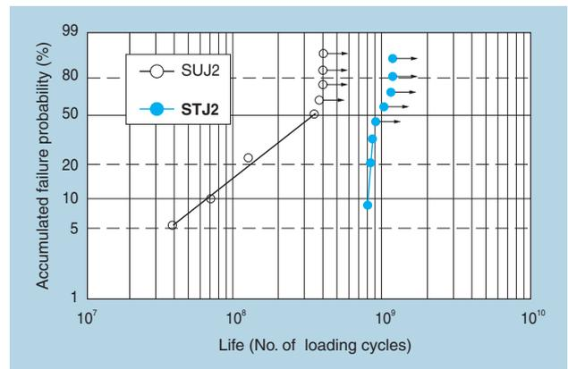
**Fig. 5** Life test result with point contact test pieces
